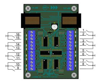
Each terminal block with 3 pole contains two input terminals and one terminal connected to Common/"C". These Common/"C" terminals are internally connected to circuit ground. We recommend using isolated external contacts (open-collector/drain outputs, relay contacts) for driving them.
