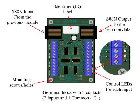
S88N modules can be numbered using a unique identifier. This identifier can be marked on the ID label located on the module.
